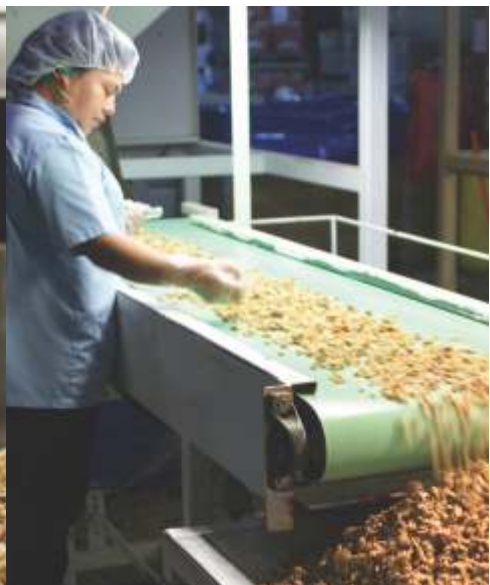
Step 6 Finally, the walnuts are inspected and hand-sorted by trained sorters to ensure they are clean and of specified color.
