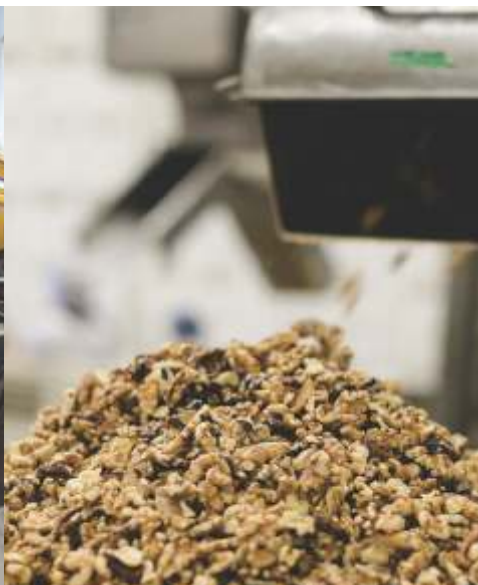
Step 5 Shelled walnuts are mechanically cracked as needed and further graded by color before kernels are screened and separated into different sizes according to USDA standards.
