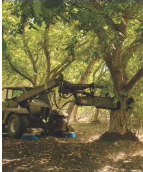
Step 1 Mechanical shakers vigorously shake each tree and thousands of walnuts fall to the ground.
