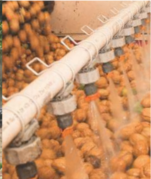
Step 3 Once walnuts are harvested, a huller removes the outer green husk. Then the walnuts are washed and dried to stabilize moisture and protect quality during storage.
